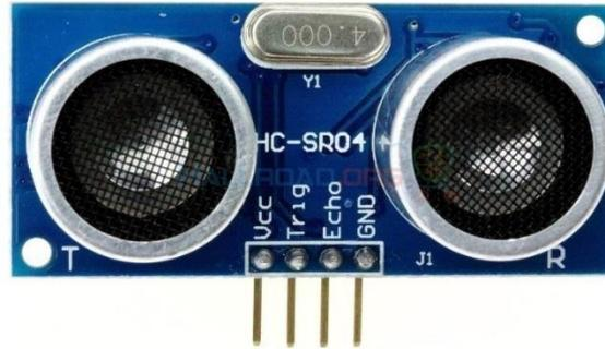
This sensor sends ultrasonic waves in the air and when these waves are hit by the object. These waves are sent back to the ultrasonic receiver module [1]. The signals are sent to the Arduino Uno which is a microcontroller board and has 14 digital input and output. The coding is through
